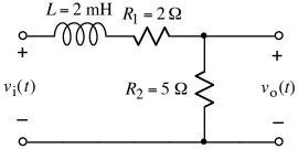
a) For the above circuit, determine the transfer function  $H(j\omega) = V_0/V_i$ .
