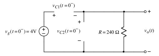
The *R* discharges  $C_2$  so all of the source voltage appears across  $C_1$ :
