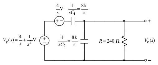
c) We sum the voltage sources and then convert the voltage sources,  $C_1$ , and  $C_2$  to a Thevenin equivalent form.
