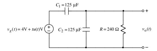
Note: The 4 V in the  $v_g(t)$  source is always on.
