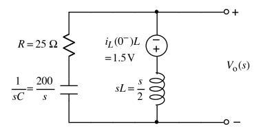
The output voltage is found by using a voltage-divider formula. We observe that  $V_0(s)$  is measured across the R and C. Thus, we may use a voltage-divider formula that avoids the need to add the voltage source to our answer. (An alternative approach is to use a voltage-divider to find the voltage across the L and then add the voltage source to our answer.)
