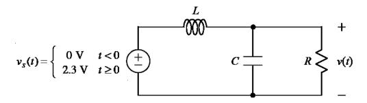
The above circuit models a digital logic gate driving another digital logic gate (modeled as R and C) via a long path of metal on-chip (modeled as L).
