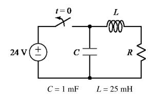
A relay is driven by a 24 V power supply, as shown above. Power is turned off at t = 0. The current, i(t), for t > 0 has two terms that decay exponentially without oscillation. One term dies out quickly, and the other term dies out with a time constant of  $\tau = 10$  ms, as in  $e^{-t/10\text{ms}}$ . Given the time constant and the information in the diagram above, find the value of *R*.
