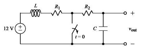
A 12 V power supply drives a long wire, (modeled as L and  $R_1$ ), followed by a short wire,  $R_2$ , and a smoothing capacitor, C. There is a safety switch, located before the smoothing capacitor, to turn off the output at the remote end. The switch is closed for a long time before opening at t = 0.
