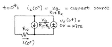
Because the C acts like a wire, all the current from the L will flow thru the C. So the current in  $R_2$  is zero. (Another way to see this is to observe that  $R_2$  has  $OV = V_C$  across it, and by Ohm's (aw  $i(O^+) = OV/R_2 = OA$ )
