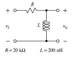
a) Determine the transfer function  $V_0/V_i$ .
