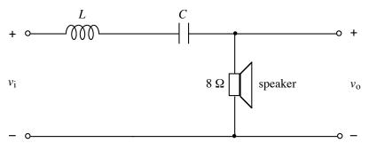
The above circuit is part of a simple crossover network for driving a midrange speaker having an impedance of  $\$\Omega$ . The circuit is described at the following web site: http://www.termpro.com/articles/xover2.html. A more in-depth discussion of crossover networks may be found at http://sound.westhost.com/lr-passive.htm.
