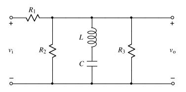
$R_1 = 18 \Omega$   $R_2 = 48 \Omega$   $R_3 = 144 \Omega$   $C = 31.25 \mu F$  L = 2 mH
