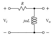
The voltage-divider formula gives the transfer function, starting with the formula for  $V_0$ :
