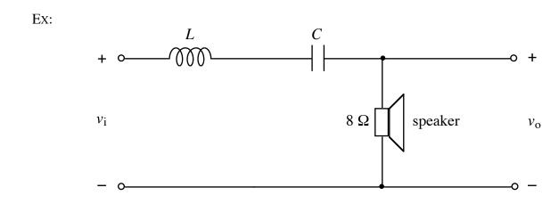
The above circuit is part of a simple crossover network for driving a midrange speaker having an impedance of  $\$\Omega$ . The circuit is described at the following web site: <u>http://www.termpro.com/articles/xover2.htm</u>]. A more in-depth discussion of crossover networks may be found at <u>http://sound.westhost.com/lr-passive.htm</u>.
