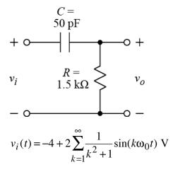
For the above circuit, determine the transfer function  $H(j\omega) = V_0/V_i$ . Assume the circuit in problem 4, has the following input signal:
