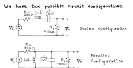
Note: R, must be to the right of L and C in order to have any effect from the L and C in the <u>series</u> configuration.
