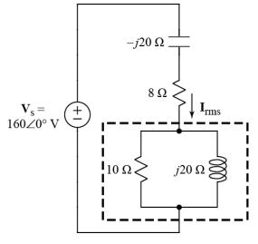
a) Calculate the value of rms current,  $\mathbf{I}_{rms}$ , flowing down through the dashed box.
