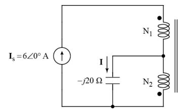
b) The turns ratio of the transformer is  $N_1/N_2 = 6$ . Calculate the numerical value of phasor current, **I**, flowing down through the capacitor. Note: the transformer is ideal.
