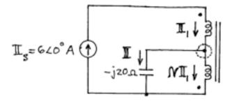
A current summation at the node with the dashed circuit, and the observation that  $II_1 = II_3$  yields the following equations:
