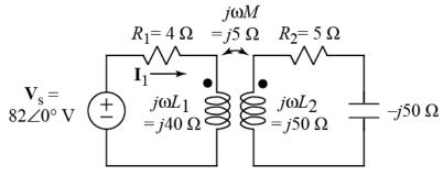
a) Calculate the numerical value of phasor current,  $I_1$ , flowing into the primary side of the transformer. Note: the transformer is linear.
