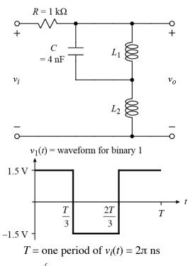
$$v_{1}(t) = \begin{cases} 1.5 \text{ V} & 0 \le t < T/3 \\ -1.5 \text{ V} & T/3 \le t < 2T/3 \\ 1.5 \text{ V} & 2T/3 \le t \le T \end{cases}$$
