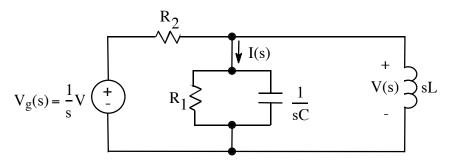
First, we find V(s). We can then find I(s) from V(s) using Ohm's law. Our calculations are cleaner if we use a Thevenin equivalent for  $V_g(s)$ ,  $R_1$ , and  $R_2$ .
