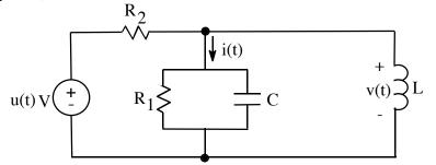
The initial energy stored in the circuit is zero.  $R_2 = 500 \Omega$  L = 200 mH
