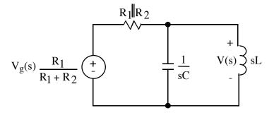
The impedance of the L and C in parallel is
