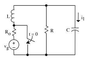
$\begin{aligned} &v_g \text{ is a dc voltage source} \\ &\text{After having been open for a long time, the switch is closed at } t=0. \end{aligned}$
