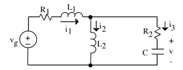
At t = 0,  $v_g(t)$  switches instantaneously from  $-v_0$  to  $+v_0$ .
