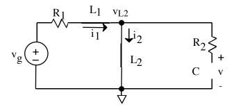
Since no current flows through  $R_2$ , we may find  $i_1$  (which equals  $i_2$ ) from the loop on the left side.
