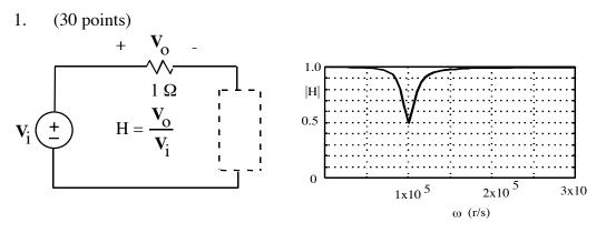
Using not more than one each R, L, and C, design a circuit to go in the dashed-line box that will produce the |H| vs.  $\omega$  shown above, that is:
