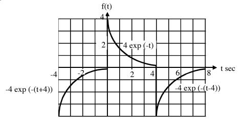
Find the coefficients for the Fourier series of the above function. The period of the function is 8 sec. From integral tables or a calculator we have:
