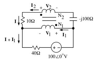
Note: We measure  $V_1$  and  $V_2$  with plus signs at dots on transformer.
