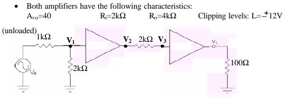
(a) Redraw this 2 stage amplifier using the amplifier model. Make sure to label  $V_1$ ,  $V_2$ ,  $V_3$ , and  $V_L$  on the schematic. (15 points)
