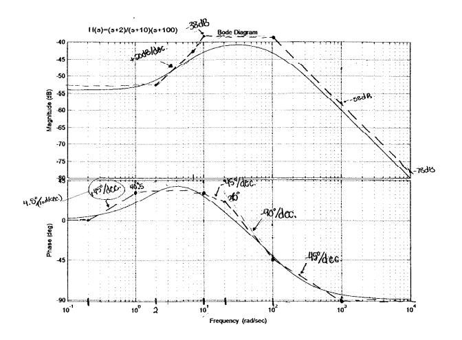
(4) b. Step 1: (starting value) remove the zero from the transfer function and find the DC gain: k=H(s); ± | = 10/(16) = 1 => OdB The start value will be 20 log. (|K,1·wstart) where n is (+)for a zero, negative for a pole. n= #of poles or zeros at s=0. L IF wstart=.01 => 20 log. (111.01)=-40dB. The line will be n x20dB/de Draw a horizontal line at o+n.90° if k>0 or 180° th.90° if K<0 K=1 : phase > 90° (n=1 for own case)
