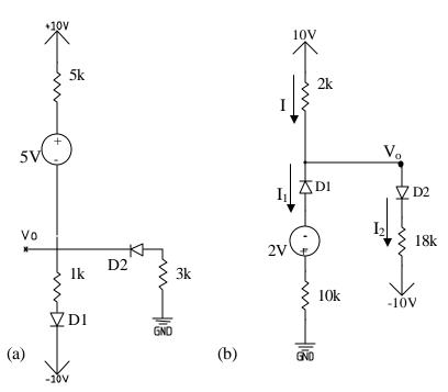
4. Assume all diodes are identical and have  $V_{DO}$ =0.7V, n=1, and  $V_{T}$ =25mV. Use the constant voltage drop method. Verify that your assumption for the diode operations(i.e. on or off) are correct. Find the following making sure you find the <u>correct</u> operation of the diodes.
