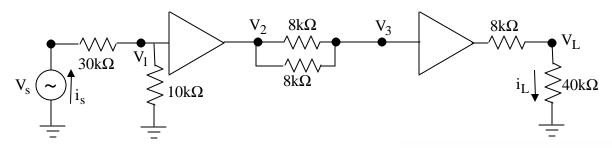
(a) Draw this 2 stage amplifier using the following model. Make sure to label  $V_S$ ,  $V_1$ ,  $V_3$ , and  $V_0$  on the schematic. Cin=3pF. Find  $V_L/V_s$  frequency response transfer function. Sketch the Bode plots using a straight line approximation and using MATLAB.
