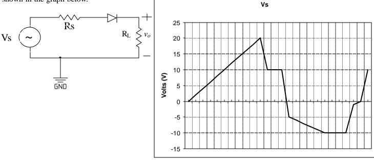
3. Use the constant voltage drop diode model with  $V_{D0}$ =0.7 to solve the circuits below for all currents in all branches of the circuit and Vo. Verify your answers.
