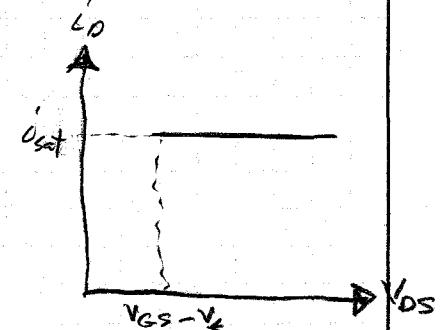
Induced Channel is uneven and "pinched off" stopping the current from increasing with the voltage.
