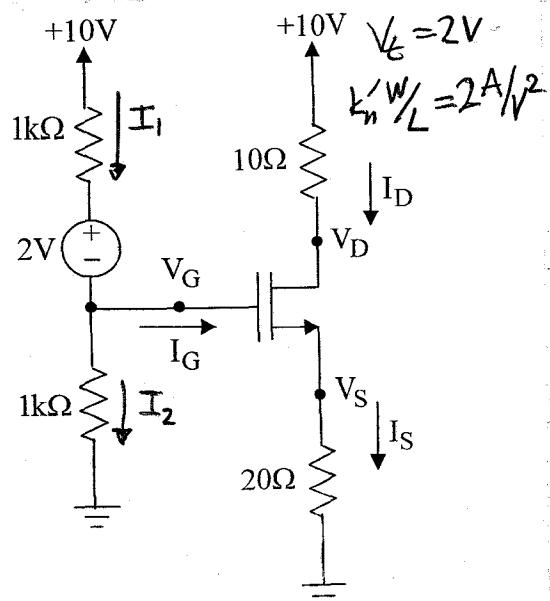
$$I_S = I_D \Rightarrow \frac{V_S}{20\Omega} = \frac{10V - V_D}{10\Omega} \Rightarrow V_D = 10V - \frac{1}{2}V_S$$
