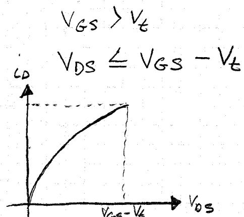
Induced channel increases at nearly the same rate in all directions with increased  $V_{DS}$  in this region. The I-V relationship is shown on the graph. It is characterized by the following equation.
