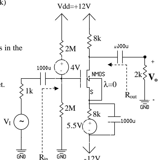
6.  $V_I$  is an AC voltage source. Use  $\lambda=0$ ,  $g_m=1\text{mA/V}^2$
