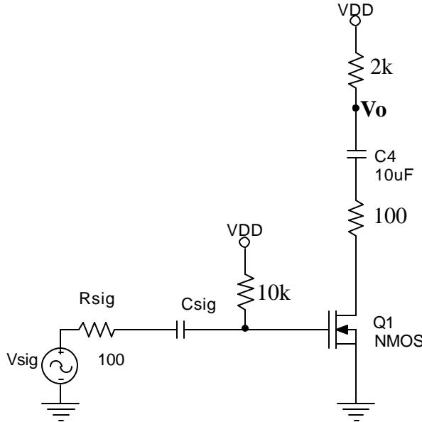
2. (a) Solve the DC circuit(schematic below) to find  $I_D$  and  $V_{GS}$  (assume caps open)
