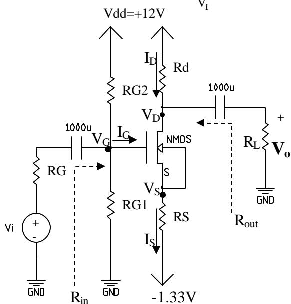
7. Use  $V_t=2\text{V}$ ,  $k_n'(W/L)=3\text{mA/V}^2$ ,  $\lambda=0$ ,  $V_s$  is an AC voltage source.  $g_m=10\text{mA/V}^2$
