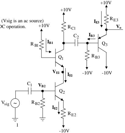
4. Use  $|V_{BE}|=0.7$ ,  $\beta=20$ ,  $V_T=25mV$  (Vsig is an ac source), ignore  $r_o$ .
