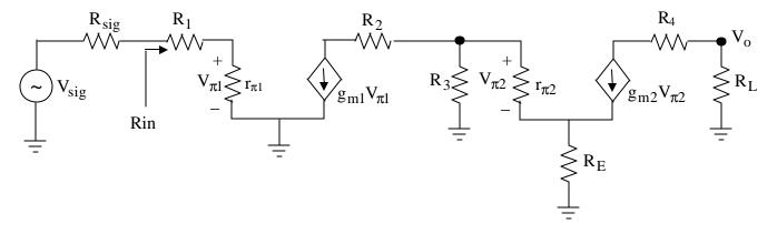
5. Use  $|V_{BE}|=0.7$ ,  $\beta=100$ ,  $V_T=25mV$  (Vs is an ac source), ignore  $r_o$ . This small-signal model comes from a circuit that has 2 transistors Q1 and Q2 denoted below as subscripts 1 and 2. It was found that  $I_{E1}=2.525m$  and  $I_{E2}=1.2625m$ . Find  $R_{in}$ (ignore Vs and  $10\Omega$ ),  $R_{out}$ (ignore  $R_L$ ), and midband gain, Vo/Vs.
