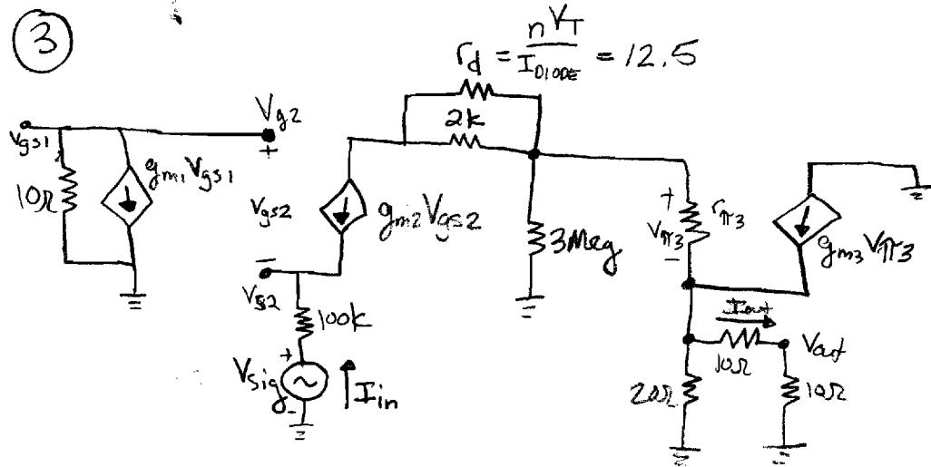
$$V_{gs1} = -g_m1 V_{gs1} \cdot 10\Omega$$
