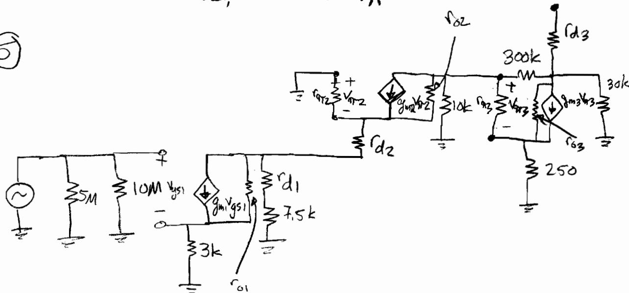
$$\textcircled{6} \quad \frac{V_{o1}}{V_4} = 83 \frac{V}{V} \quad \frac{V_{o2}}{V_{o1}} = 1 \frac{V}{V}$$
