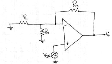
a) State the equation for Vo. Include no more than  $V_{IN}$ ,  $R_1$ ,  $R_2$ , and  $R_3$ .
