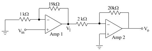
Modify the above circuit to compensate for input bias current on both amplifiers.
