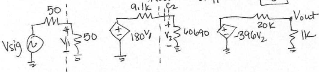
$$\frac{V_{out}}{V_{sig}} = \frac{-396(1k)}{21k} \cdot \frac{180(60,690)}{(60,690 + 9.1k)} \cdot \frac{50}{100} = -1,476 \text{ V/V}$$
