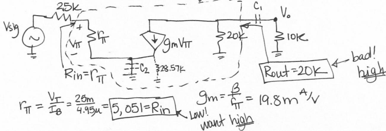
$$r_\pi = \frac{V_T}{I_B} = \frac{25m}{4.95\mu} = 5,051 = R_{in}$$
