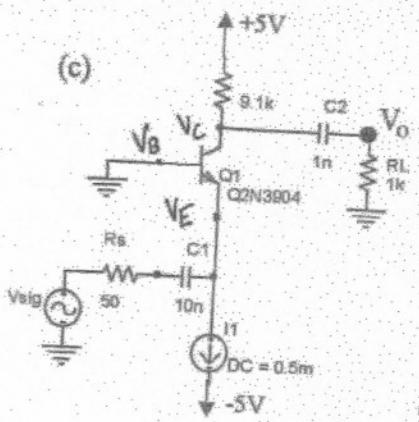
$$\begin{aligned}I_E &= 0.5 \text{ mA} \\I_C &= 0.495 \text{ mA} \\I_B &= 4.95 \mu\text{A}\end{aligned}$$
