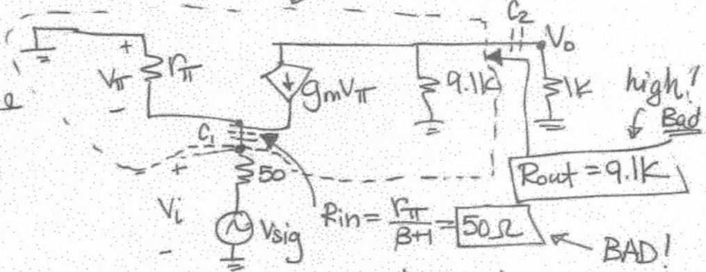
$$r_{\pi} = \frac{25 \text{ m}}{4.95 \mu\text{A}} = 5.051 \text{ k}\Omega$$
