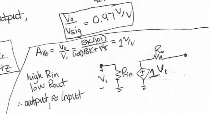
$$A_{vo} = \frac{V_o}{V_i} = \frac{13k(101)}{(101)13k + r_\pi} = 1V/V$$
