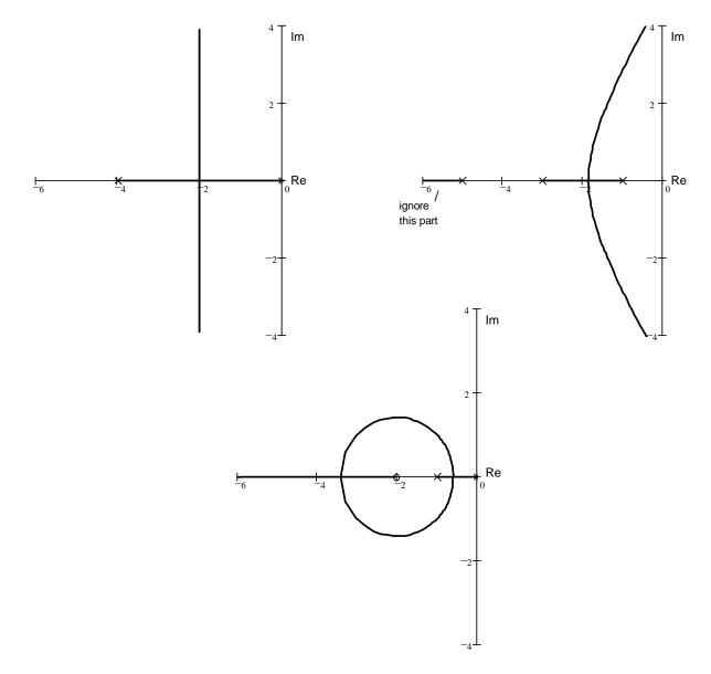
b) Assuming you can tolerate about 4% overshoot (  $\zeta = .707$  ) in the step response and that the speed of response will increase with a little ringing, estimate the best position for the closed loop pole(s). Label that (or those) position(s) with the letter "b".
