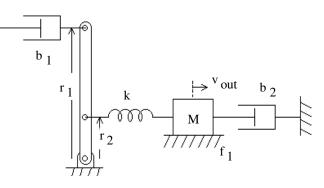
2. Find the equivalent electric circuit for the mechanical system shown.  $\omega_{in}$  is the input.
