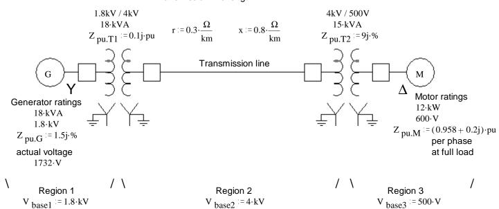
Set the  $V_{base}$  values in each region by looking at the transformer ratings.
