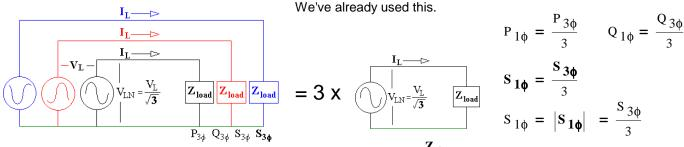
Anything not Y-connected can be converted to a Y- equivalent.  $\mathbf{Z}_{\mathbf{Y}} = \frac{\mathbf{Z}_{\Delta}}{3}$
