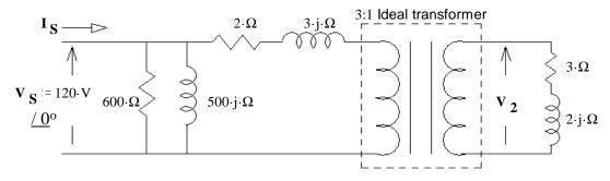
b) Find the secondary voltage. Magnitude only.  $|V_2| = ?$
