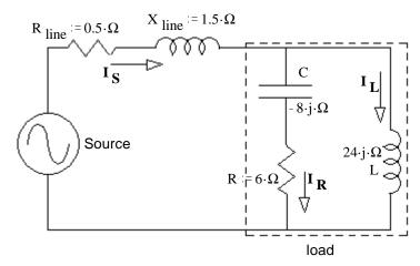
b) The voltage at the load (magnitude).  $V_{Load} = ?$
