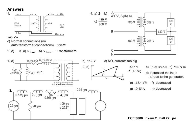
3. (18 pts) A one-line, per-phase diagram is shown below. Using the S<sub>base</sub> given, draw a per-phase, per-unit diagram. Include pu values for <u>all</u> the values given in the drawing below. E<sub>A</sub> voltage is line-to-neutral.
