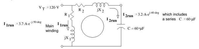
a) Find the run-speed impedances of winding 1 and winding 2 without the capacitor. Find both in rectangular form.
