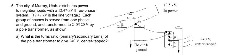
b) When a 1500-W toaster-oven is turned on, how much does the current increase in the high-voltage wire? Assume the power factor is unity and the transformer is 100% efficient.
