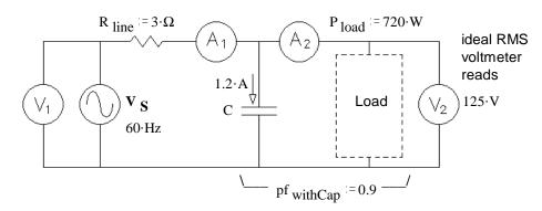
b) The load can be modeled as 2 parts in series. Draw the model and find the values of the parts.
