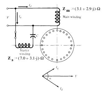
8. A 1/3-hp, 120-V, 60-Hz, single-phase, capacitor-run, single-phase induction motor has two identical windings Ind3 p5 set 90° apart in the motor housing. Each winding draws 6.8 A at 20° lag when the rotor is locked and 2 A at 40° lag when the motor is running at its rated speed. This is with no added capacitors, so the motor would have to be started by hand.
