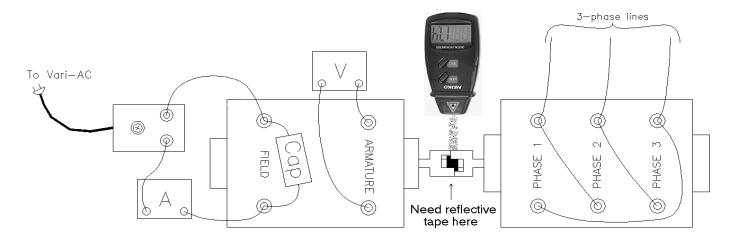
maximum. If the speed seems unreasonable high (above 1800rpm), hold the tachometer further away from the spinning coupling. Now that you have the DC motor spinning at a reasonably constant speed, you can get data to plot a curve like that shown in Figure 8-30 (p.398) of your textbook.
