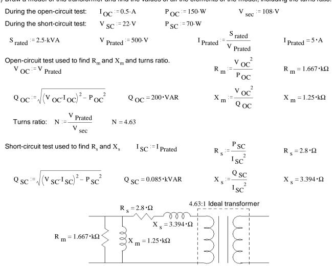
b) The transformer is connected to a primary source voltage of 360V and loaded with  $\mathbf{Z}_{\mathbf{L}} := (2 + 1 \cdot \mathbf{j}) \cdot \Omega$ Find the secondary voltage. Magnitude only.  $|\mathbf{V}_{2}| = ?$
