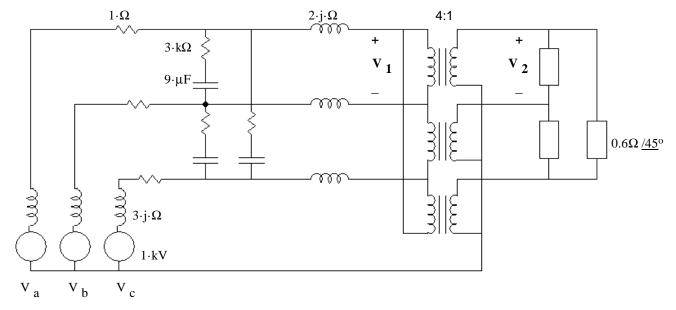
b) Find  $\frac{V_1}{V_2}$  including phase angle
