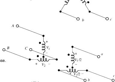
7. A phase-shifting transformer has a complex turns ratio of  $\mathbf{t} := 4 \cdot e^{\mathbf{j} \cdot 20 \cdot \deg} = 4 \cdot \underline{/20^{\circ}}$  It has a series impedance of  $\mathbf{Z}_{\mathbf{S}} := (0.05 + \mathbf{j} \cdot 0.6) \cdot \Omega$  Find the admittance matrix of this transformer (see the last page of the transformer notes).
