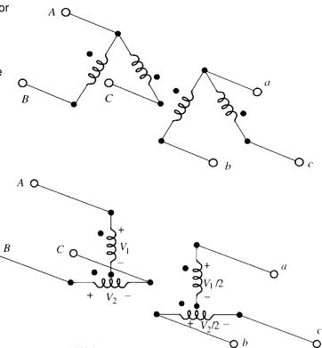
7. A phase-shifting transformer has a complex turns ratio of  $t = 4 \cdot e^{j \cdot 20 \cdot deg} = 4 / 20^{\circ}$
