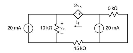
Find  $v_x$ ,  $i_1$ , and the power dissipated by the dependent source.
