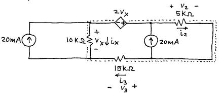
Second, write v-loop eghs for loops not containg current src15. There is only one such loop, indicated by the dotted line:
