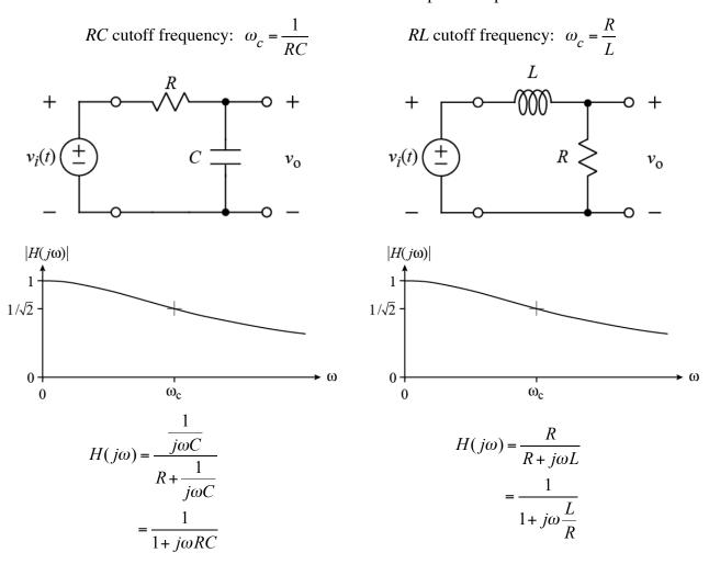
**TOOL:** The *RC* and *RL* circuits shown below act as one-pole low-pass filters.
