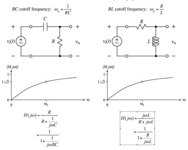
**TOOL:** The *RC* and *RL* circuits shown below act as one-pole high-pass filters.
