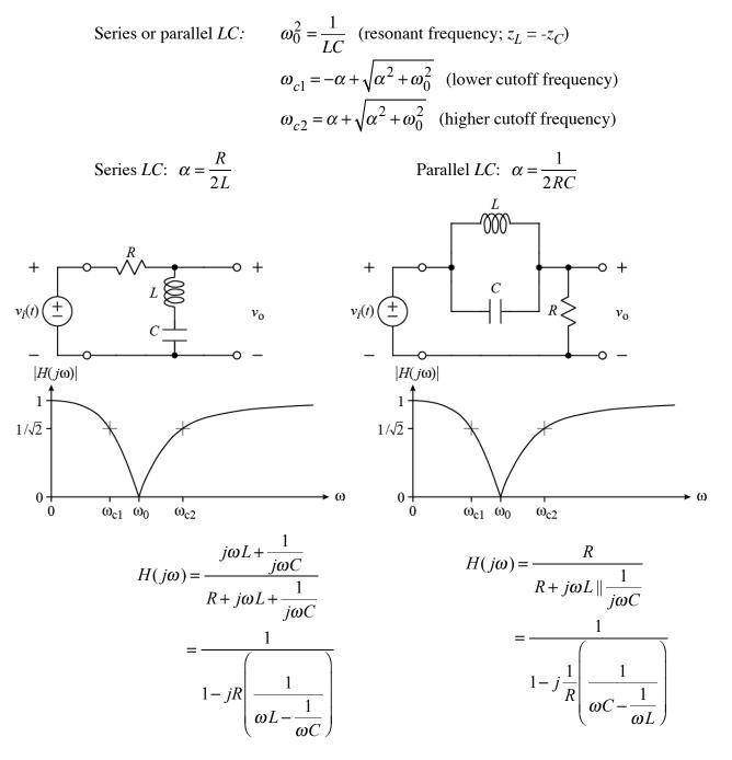
Fig. 1. Series *LC* band-reject filter.
