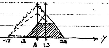
The center of mass lies at  $y = 1.3$  since the centroid for  $y_{11}$  has zero area or mass and  $y_{32}$  centroid has nonzero area.
