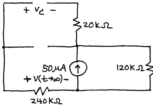
No current can flow thru the  $240\text{ k}\Omega$  resistor.
