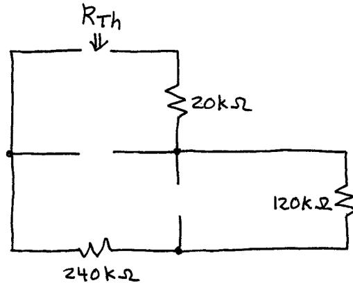
$$R_{Th} = 20\text{k}\Omega + 120\text{k}\Omega + 240\text{k}\Omega = 380\text{k}\Omega$$
