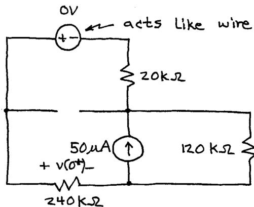
This is a current-divider circuit with  $20\text{k}\Omega + 240\text{k}\Omega = 260\text{k}\Omega$  on one side and  $120\text{k}\Omega$  on the other side.
