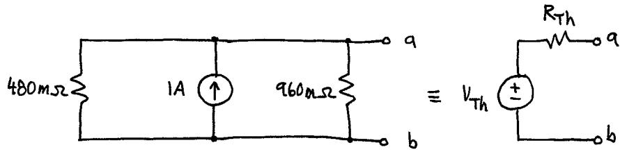
$V_{Th} = V_{a,b}$  with nothing attached to  $a, b$ .
