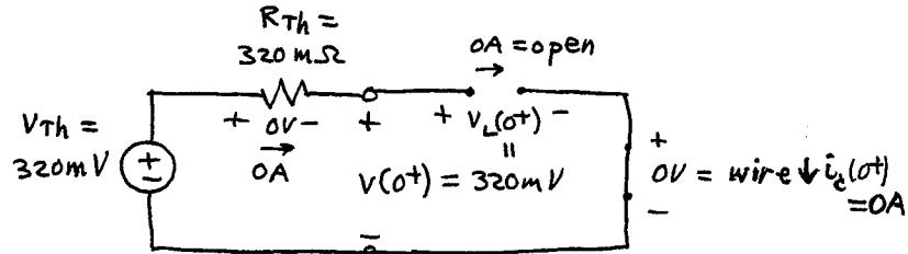
$$v(0^+) = 320\text{mV} \text{ from above circuit}$$
