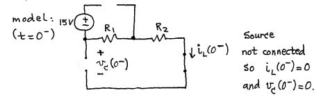
Fourth, we have  $i_{L}(0^{+}) = i_{L}(0^{-})$  and  $v_{C}(0^{+}) = v_{C}(0^{-})$  since these are energy variables  $(w = \frac{1}{2}Li^{2})$  and  $w = \frac{1}{2}Cv^{2}$  that cannot change instantly.
