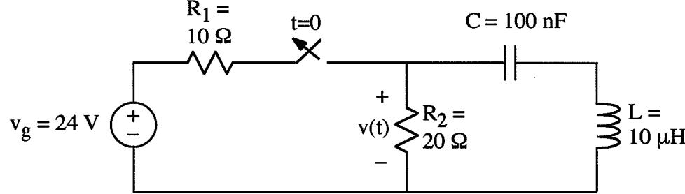
After being closed for a long time, the switch opens at  $t = 0$ .
