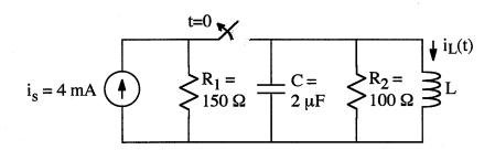
After being closed for a long time, the switch opens at t = 0.
